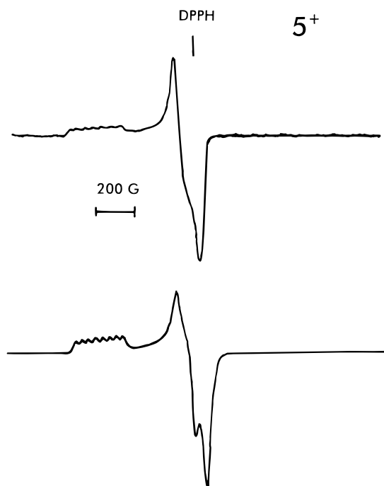
Figure 3. ESR spectrum of complex 5^+ in 1:1 \text{CH}_2\text{Cl}_2/\text{C}_2\text{H}_4\text{Cl}_2 at 77 K (top) produced by the electrolytic oxidation of 5 . The simulation shown below is based on the spectral parameters of Table 2.
